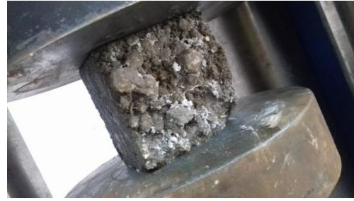
Fig. 6. Testing of the concrete cube for its compressive strength
