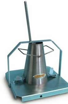
Fig. 2. Slump test using standard slump cone
